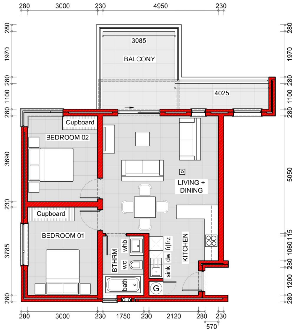
2ND FLOOR FLOOR PLAN UNIT 14 SCALE 1:100
