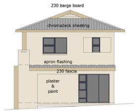
NORTH WEST ELEVATION 1:100
